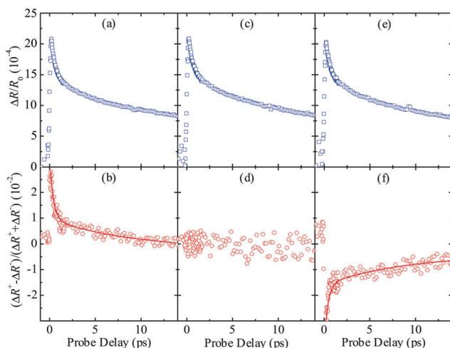
**Fig. 3** Differential reflection (a, c, e) and the ratio between difference and sum of the two circular components (b, d, f) of monolayer MoSe<sub>2</sub> measured with pump pulses of  $\sigma^+$  (a, b),  $x$  (c, d), and  $\sigma^-$  (e, f) polarizations, respectively.
