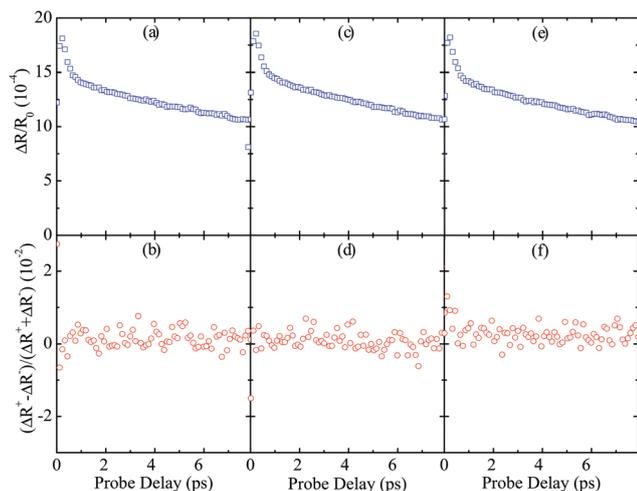
**Fig. 5** Differential reflection (a, c, e) and the ratio between difference and sum of the two circular components (b, d, f) of a few-layer MoSe<sub>2</sub> flake with pump pulses of  $\sigma^+$  (a, b),  $x$  (c, d), and  $\sigma^-$  (e, f) polarizations, respectively.
