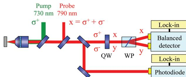
Fig. 2 Polarization-resolved differential reflection setup to measure pump-induced circular dichroism, which reflects spin and valley dynamics of excitons (QW: quarter-wave plate, WP: Wollaston prism).
