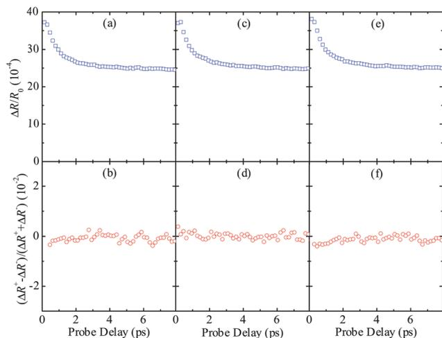
**Fig. 4** Differential reflection (a, c, e) and the ratio between difference and sum of the two circular components (b, d, f) of bulk MoSe<sub>2</sub> measured with pump pulses of  $\sigma^+$  (a, b),  $x$  (c, d), and  $\sigma^-$  (e, f) polarizations, respectively.
