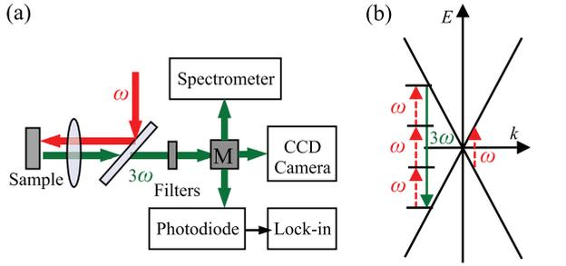
FIG. 1. (Color online) (a) Experimental schematic: A fundamental ( $\omega$ , red) pulse is normally incident on the sample. The third harmonic ( $3\omega$ , green) is detected in the reflected direction by a CCD camera, a spectrometer, or a photodiode connected to a lock-in amplifier. (b) Schematic diagram showing the linear dispersion of graphene, indicating the one-photon absorptions of  $\omega$  and  $3\omega$  and illustrating the energy level description of third harmonic generation.
