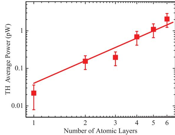
FIG. 3. (Color online) The average power of the third harmonic as a function of the number of atomic layers for an average fundamental power of 1 mW (solid squares). The solid line is a quadratic fit ( $\chi^{(3)} = 0.8 \times 10^{-16}$   $\text{m}^2/\text{V}^2$ ) of Eq. (1) to the data using parameters appropriate for our experimental conditions, as discussed in the text.
