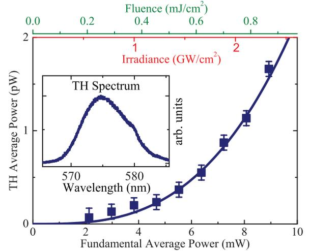
FIG. 2. (Color online) The average power of the third harmonic as a function of the average power of the incident fundamental (solid squares), and the spectrum of the third harmonic (solid squares, inset). The solid line is a cubic fit ( $\chi^{(3)} = 0.4 \times 10^{-16} \text{ m}^2/\text{V}^2$ ) of Eq. (1) to the data using parameters appropriate for our experimental conditions, as discussed in the text.
